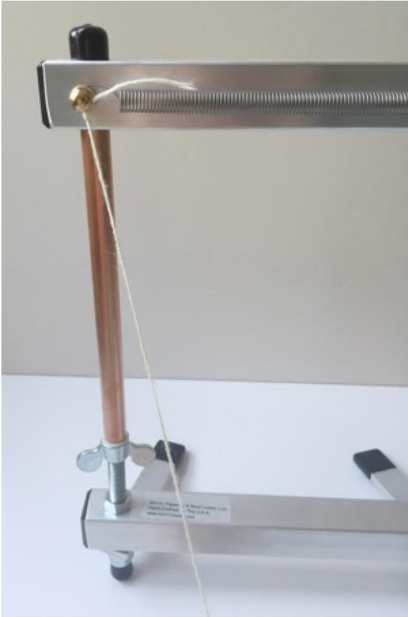
Begin warping by tying your warp material to the brass screw in the upper left corner of the loom. Bring the warp down the front of the loom, under it and up the back.
